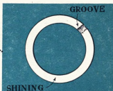
Fig. 2. Top view of imperfect seat.
